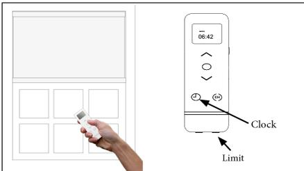
1. Push and hold the LIMIT button. While holding the limit button, push the CLOCK button for 3 seconds and release. The hour digits will flash.
