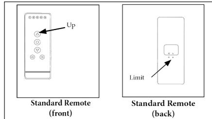
2. To save the Favorite position, hold the LIMIT button and hold the UP button at the same time. Release after a series of short beeps.
