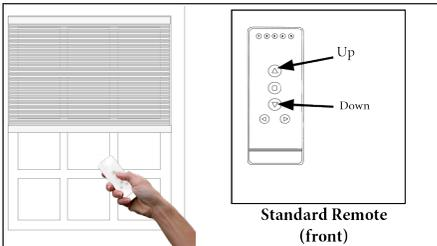
1. Using the UP and DOWN arrows, move the blind to the desired Favorite position.
