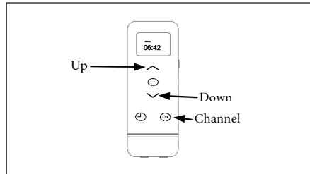
2. Use the UP and DOWN buttons to set the current hour. Press the CHANNEL button to confirm hour and advance to minutes.
