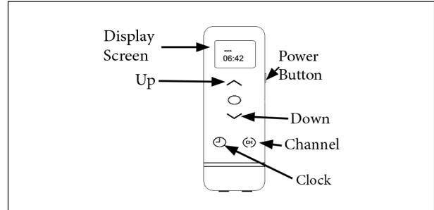
2. Your blind is now ready! Press the CLOCK button until the display shows 'Manual'. Select the programmed channel and use the UP and DOWN arrows to operate the blind.
