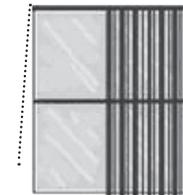
Split Draw = vanes stack equally on both sides of the headrail. Controls can be on the left or the right.
