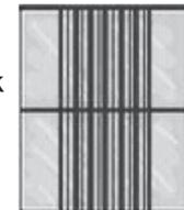
Off-Center Draw = Vanes stack unequally on both sides of the headrail, distance of draw is limited to the short side.
