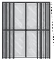
Reverse Center Draw = vanes stack to the center of the headrail. Control can be on the left or the right.
