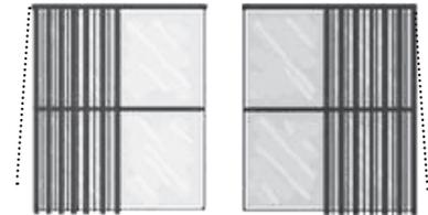
Reverse One-way Draw = controls are on the opposite side of the headrail from the stack.
